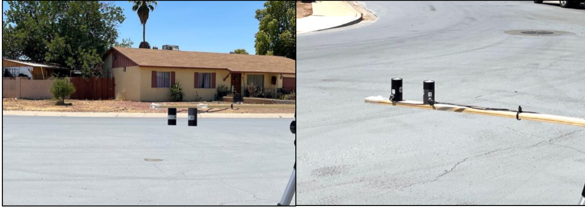
Figure 14: UVI and UVB sensors pointed up and down to determine the surface reflectivity over the CoolSeal. The same process was repeated over asphalt and concrete on June 13 th , 2022, between 12:30 pm and 1:30 pm local time.
