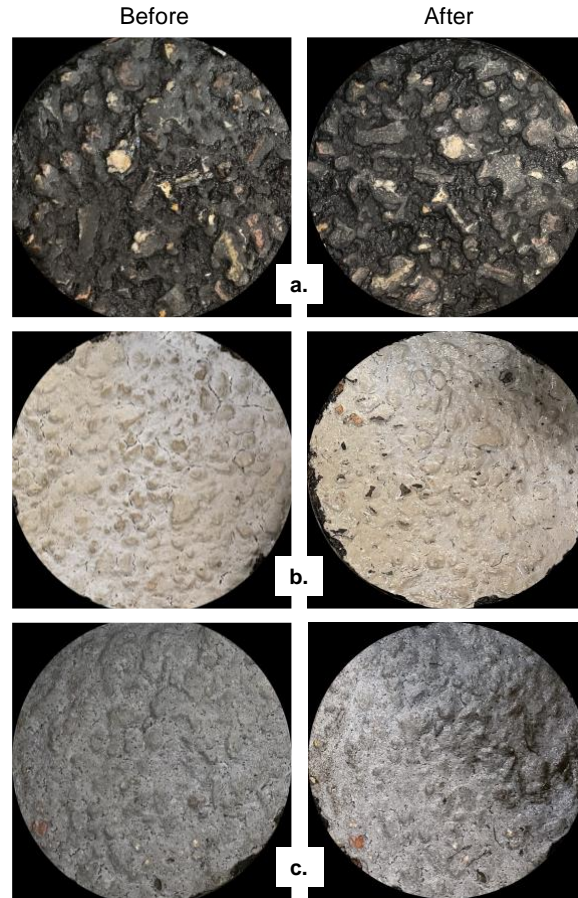
Figure 37. Field samples before and after the wear test. a. Control, b. CP-A; c. CP-B.
