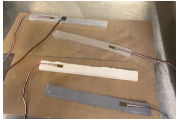
Figure 40. Expansion and Contraction Testing Samples.
