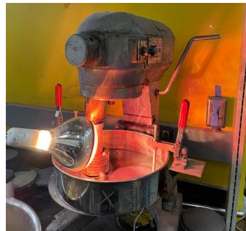
Figure 34. 250-watt heat lamp pointing to the samples during the test.
