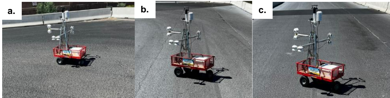
Figure 15. MaRTy at the Union Hills Service Center in Northern Phoenix during measurements on September 17, 2022, on a. the Control surface; b. the CP-A surface; and c. the CP-B surface.
