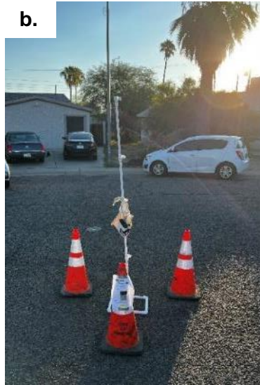
Figure 6a. Stationary RTD air temperature array over the CoolSeal in the cul de sac of W Earll Dr; and, b. the traditional asphalt in the cul de sack of W Verde Ln.
