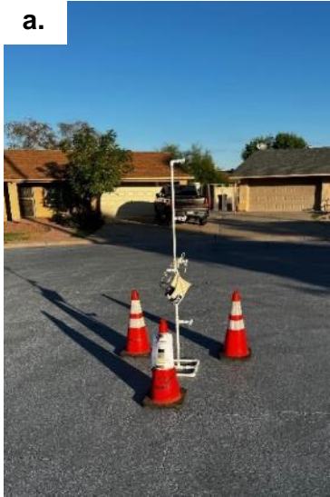
Figure 6a. Stationary RTD air temperature array over the CoolSeal in the cul de sac of W Earll Dr; and, b. the traditional asphalt in the cul de sack of W Verde Ln.
