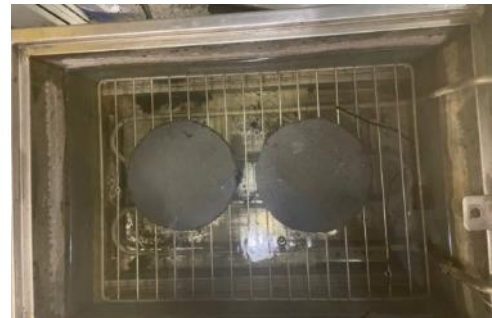
Figure 33. Samples being conditioned in the water bath at 140°F.
