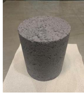
Figure 27. Gyratory plug preparation before placing it in the oven for aging.
