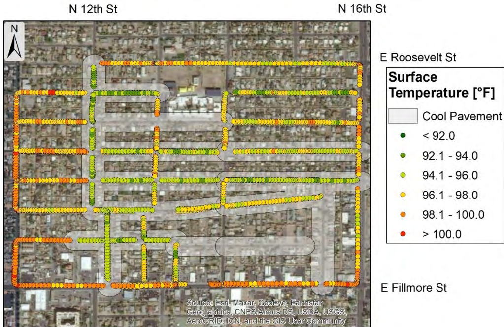
Figure A1. Map of measured and time-detrended surface temperature for 4:50 AM on August 18, 2020, in the Garfield neighborhood in district 8.
