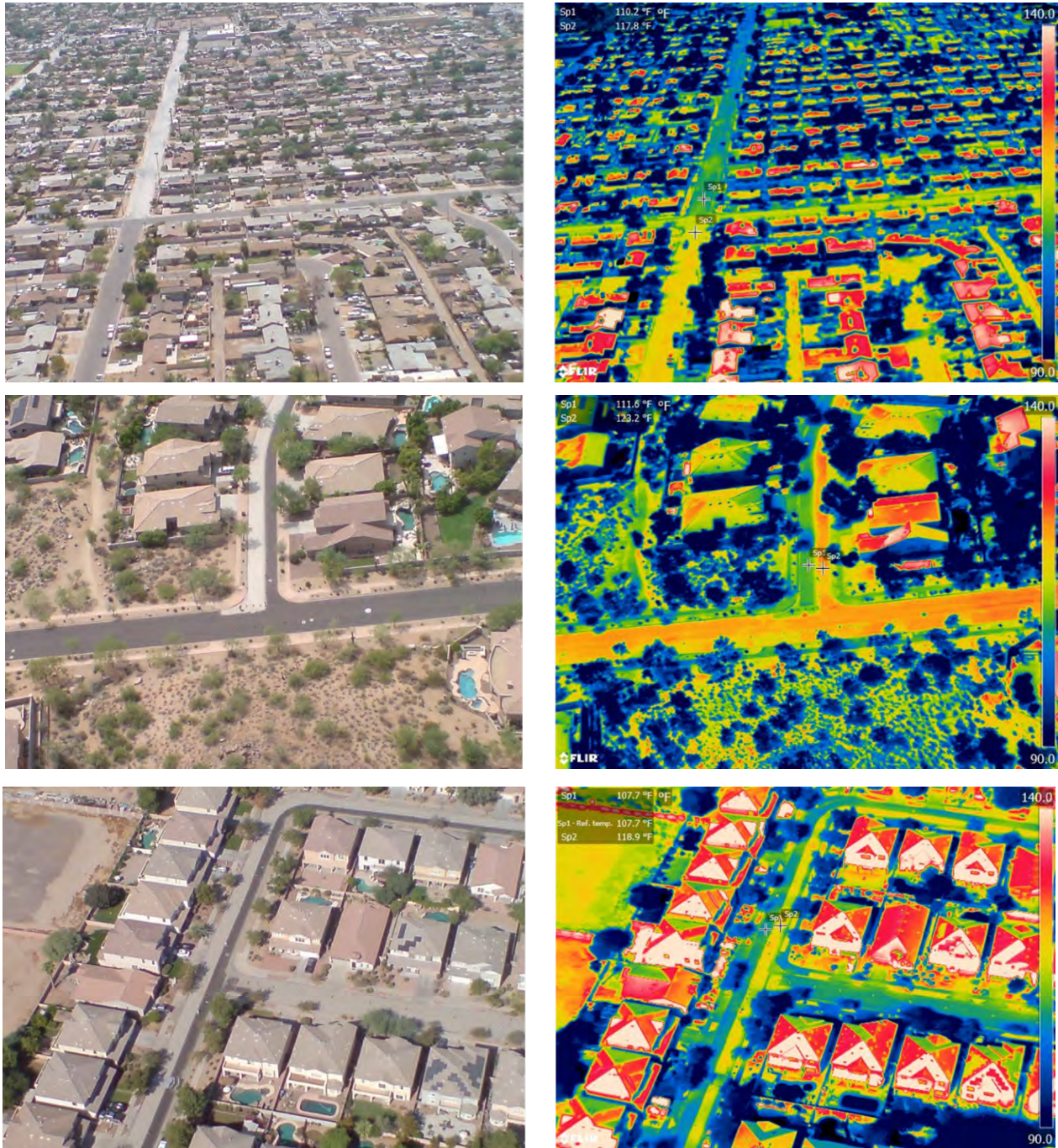
Figure 8: Side-by-side digital camera and infrared images of several locations where Cool Pavement was applied from Sept 10, 2020, 12:45pm (top), Sept 10, 2020, 1:08pm (middle), and Oct 21, 2020, 1:12pm (bottom).
