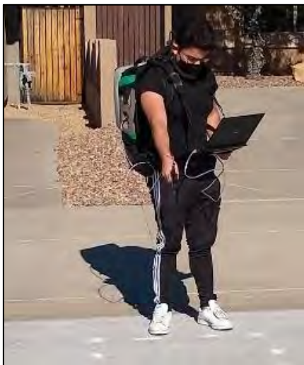
Figure 4: Surface reflectivity measurements of Cool Pavement with a spectroradiometer.
