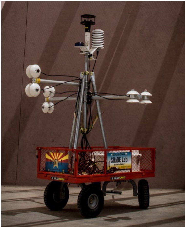
Figure 2: MaRTy, the biometeorological weather station.
