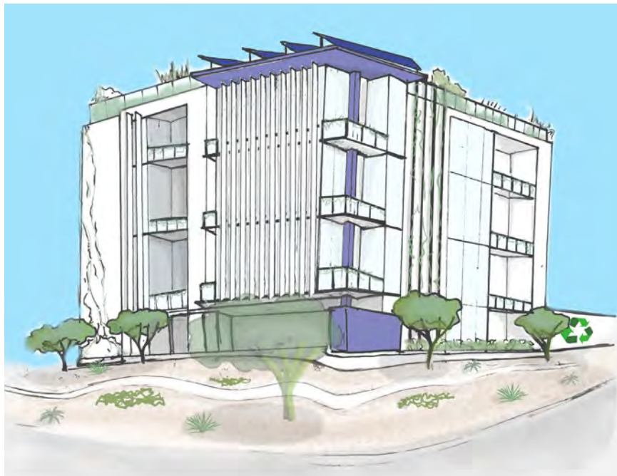
Figure 13. In this masterplan highlighting water conservation, multi-family residential housing would have rainwater harvesting, bioswales (which are landscaping elements designed to naturally filter pollution out of surface runoff), native plants, and would harvest condensate from large air conditioning units. Its no-curb system, which means it does not have raised curbs around paved areas, allows rainwater to run into landscaped or natural areas. (Katherine Keane, Superstition Studios, page 2-66).
