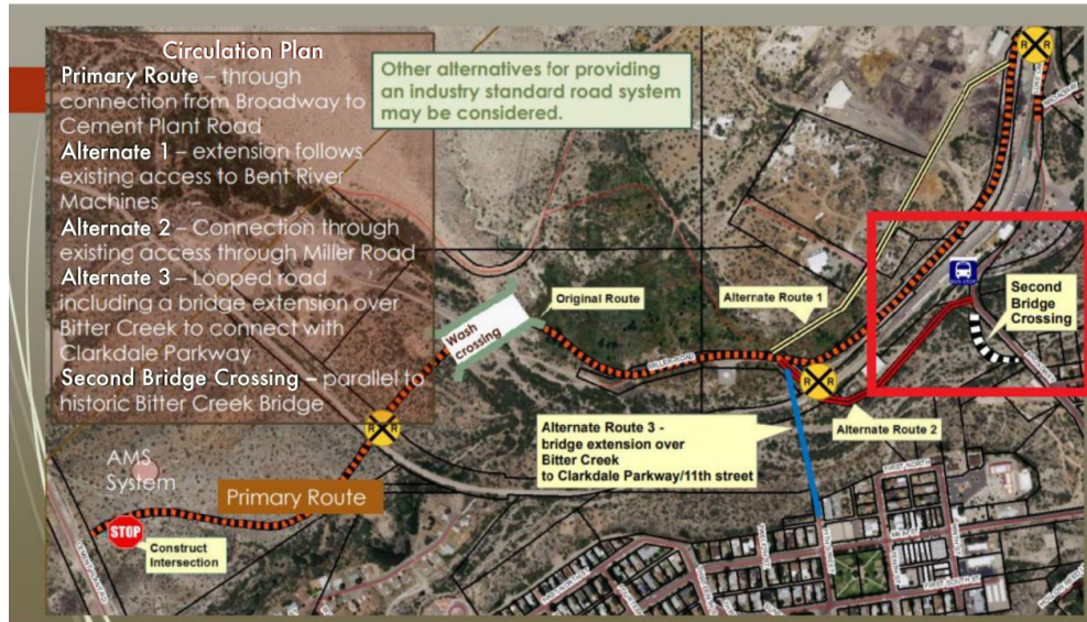
Figure 16 Annotated Bitter Creek Bridge area map, highlighting suggested alternate routes and added structure placements
