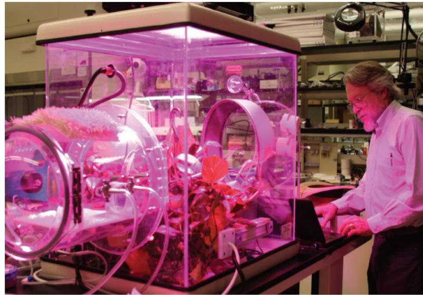
*In the laboratory, lead engineer and CNCE executive director Allen Wright monitors the carbon dioxide and atmospheric conditions to optimize plant growth and test the moisture swing sorption technology. Photo: Michelle Saldana, Biodesign Institute*
