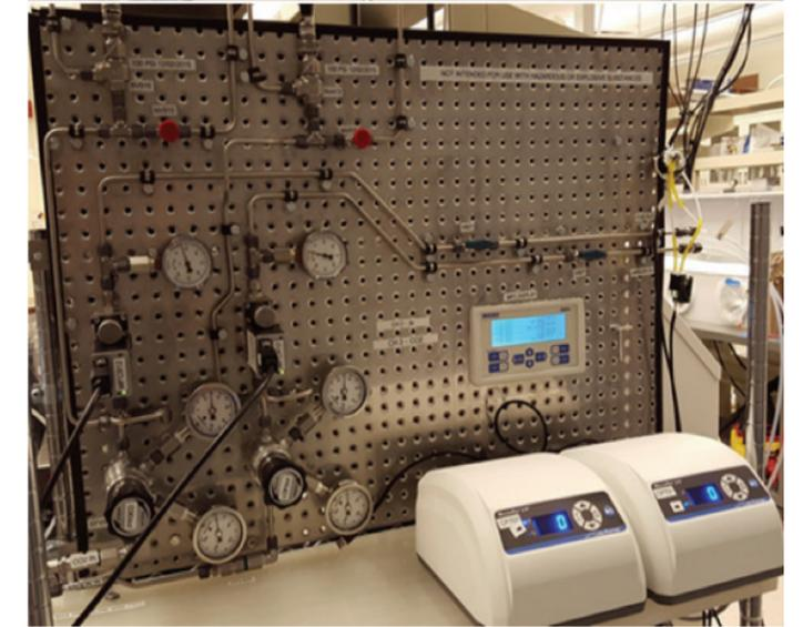
*Upper: Flow cell system for CO<sub>2</sub> separation using ionic liquids. Lower: Gas handling and controller functions for flow cell system.*
