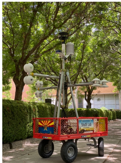
Figure 3.10: The portable MaRTy cart used for collecting microclimate data along urban transects (see Middel et al. 2019 for details).
