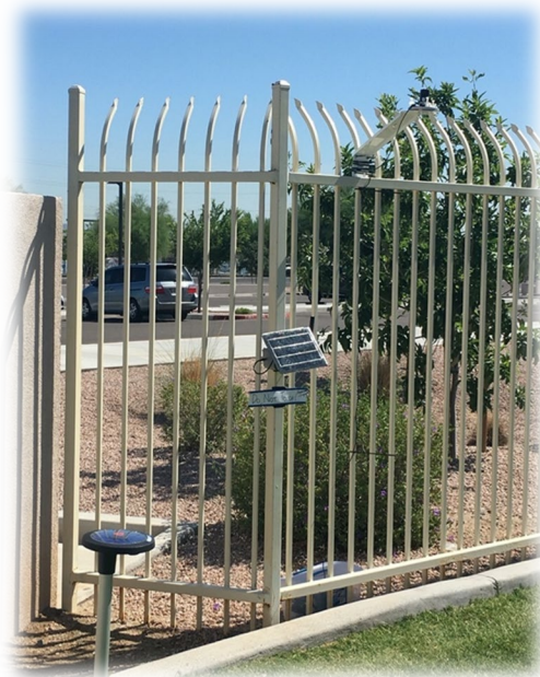
Figure 2.20. Microclimate and air quality sensors installed at Paideia Academies
