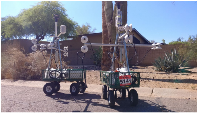
Figure 2.17. Left: MaRTy visits a PASS neighborhood. Right: Mean radiant temperature (MRT) measurements captured with MaRTy in a PASS neighborhood, fall 2019.
