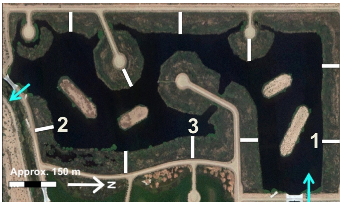
Figure 2.3: The Tres Rios CTW showing the 10 marsh transects (in white), those where water quality is also sampled (white numbers), and the inflow and outflow (blue arrows; Childers in review).
