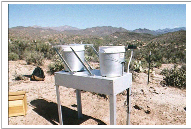
Figure 10. LTER deposition bucket collectors.
