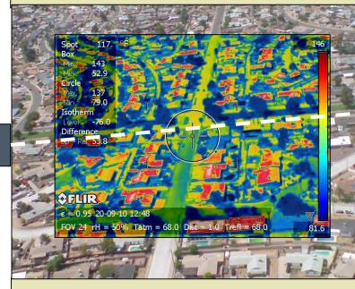
Visible and thermal images from the helicopter. Red (blue) colors indicate hotter (colder) surface temperatures relative to the temperature range in the image. CoolSeal was applied below white dashed line.
