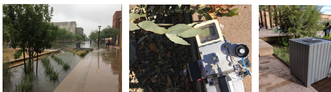
Figure 4. Site photos. Left Photograph: Bioswale at Orange Mall during October 2018 storm event. Middle photograph: IRGA being used to measure transpiration rates of Simmondsia chinensis . Right Photograph: ISCO installation with enclosure installed at Orange Mall.
