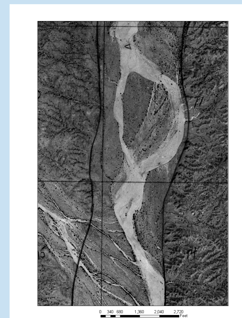
Between 1953 and 1992 the mainstem channel changed shape and width due to precipitation events. Note that southwestern and northeastern tributaries have also changed.
