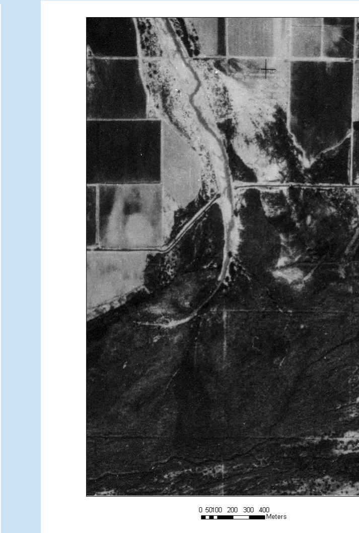
At the confluence of the Hassayampa and Gila Rivers, the channel form of the Hassayampa has changed from braided and sinuous to straight, narrow, and more vegetated to the south, 1934-1972.
