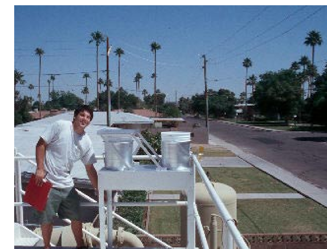
One of the AeroChemetrics wet/dry bucket collectors used by CAP LTER to directly measure deposition, at Site 1 near downtown Phoenix
