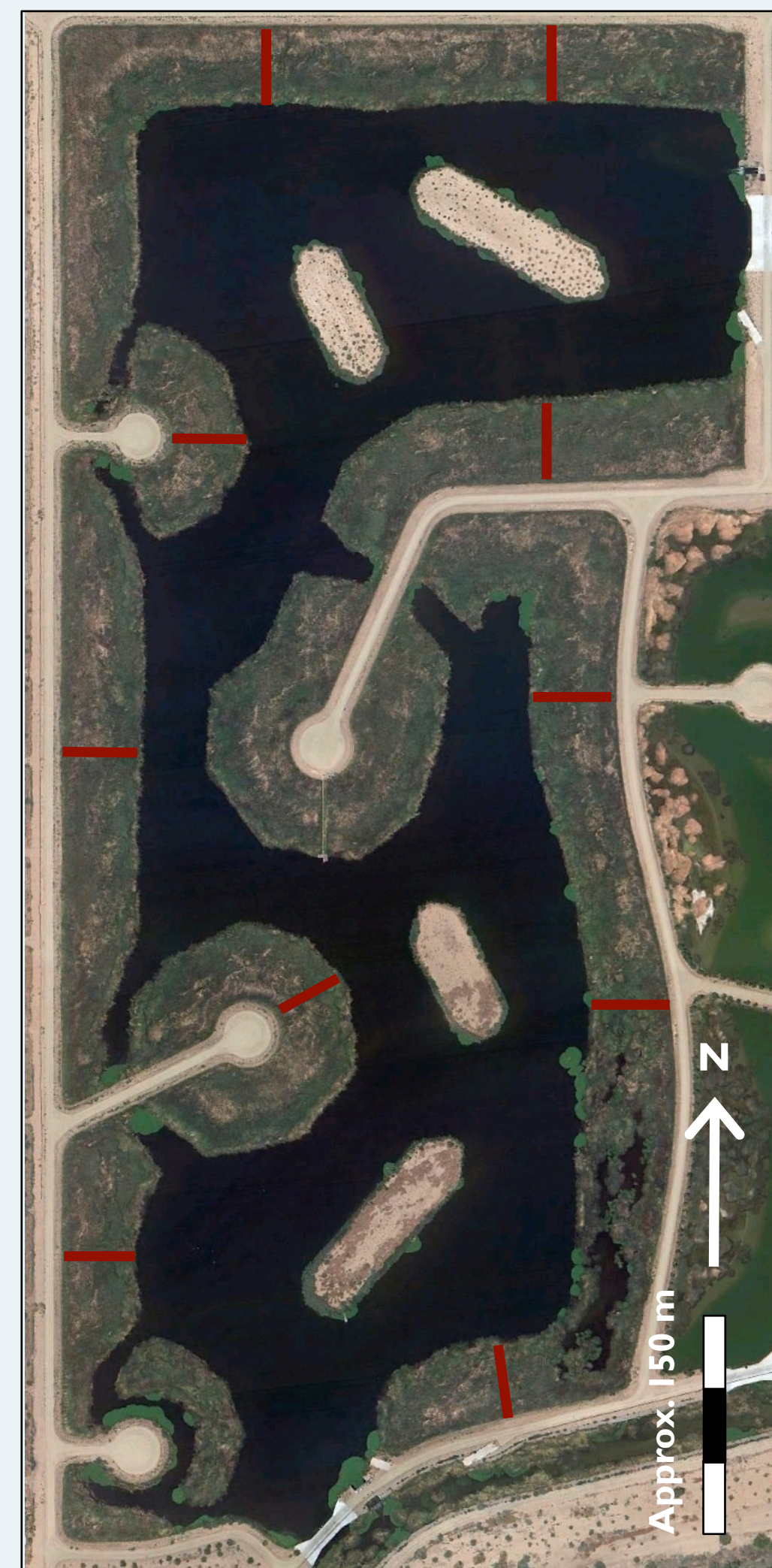
Figure 2. Constructed wetland study cell with approximate locations of 10 bimonthly sampled transects (denoted by red lines).
