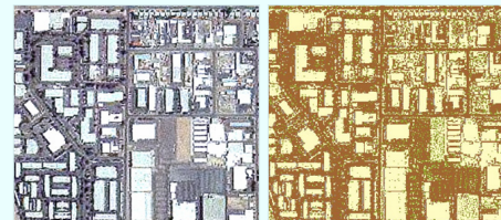
Figure 3. A sample site of mixed industrial-commercial landscape from the digital image (left) with 90.78 % TISC; the classified land cover results (right): ISC-I (brown color) = 51.54 %, ISC-II (yellow color) = 39.24 %. The green color areas are pervious surface.
