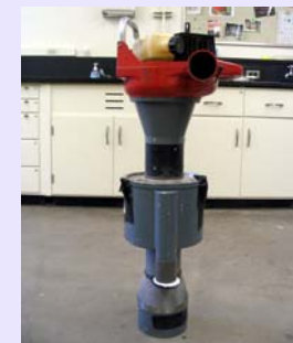
Arthropod vacuum sampler
