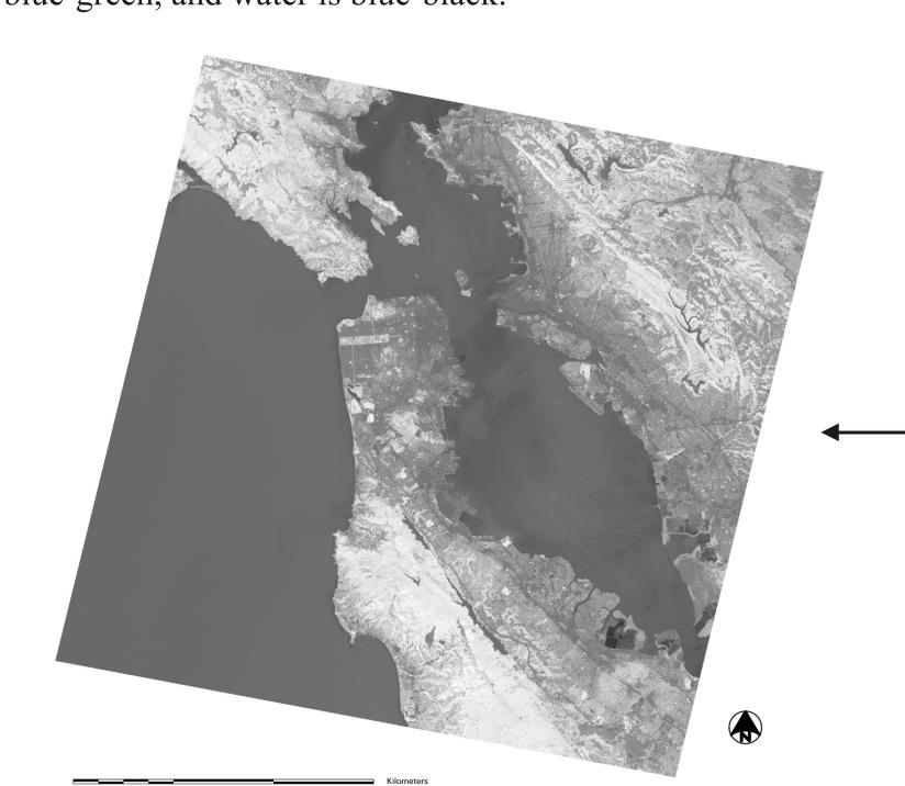
Figure 2. NDVI (Normalized Difference Vegetation Index) data derived from the visible-near infrared ASTER data in Fig. 1. Brightness corresponds to vegetation abundance (bright = high, dark = low).
