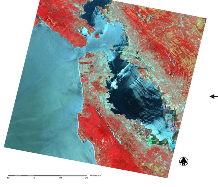
**Figure 1**. ASTER visible-near infrared (321 RGB) scene of the San Francisco metropolitan area acquired 14-June-00. Vegetation is red, urban areas are blue-green, and water is blue-black.
