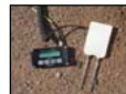
Figure 3. Field Scout TDR 100 Soil Moisture System, Spectrum Technologies (Plainfield, IL). Image captured by Catherine Singer during June 2005.
