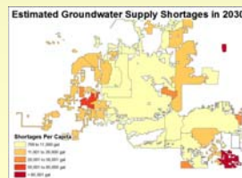
Based on the above assumptions, expected groundwater shortages by 2030 as a result of population increases and compliance with the GMA safe yield limits
