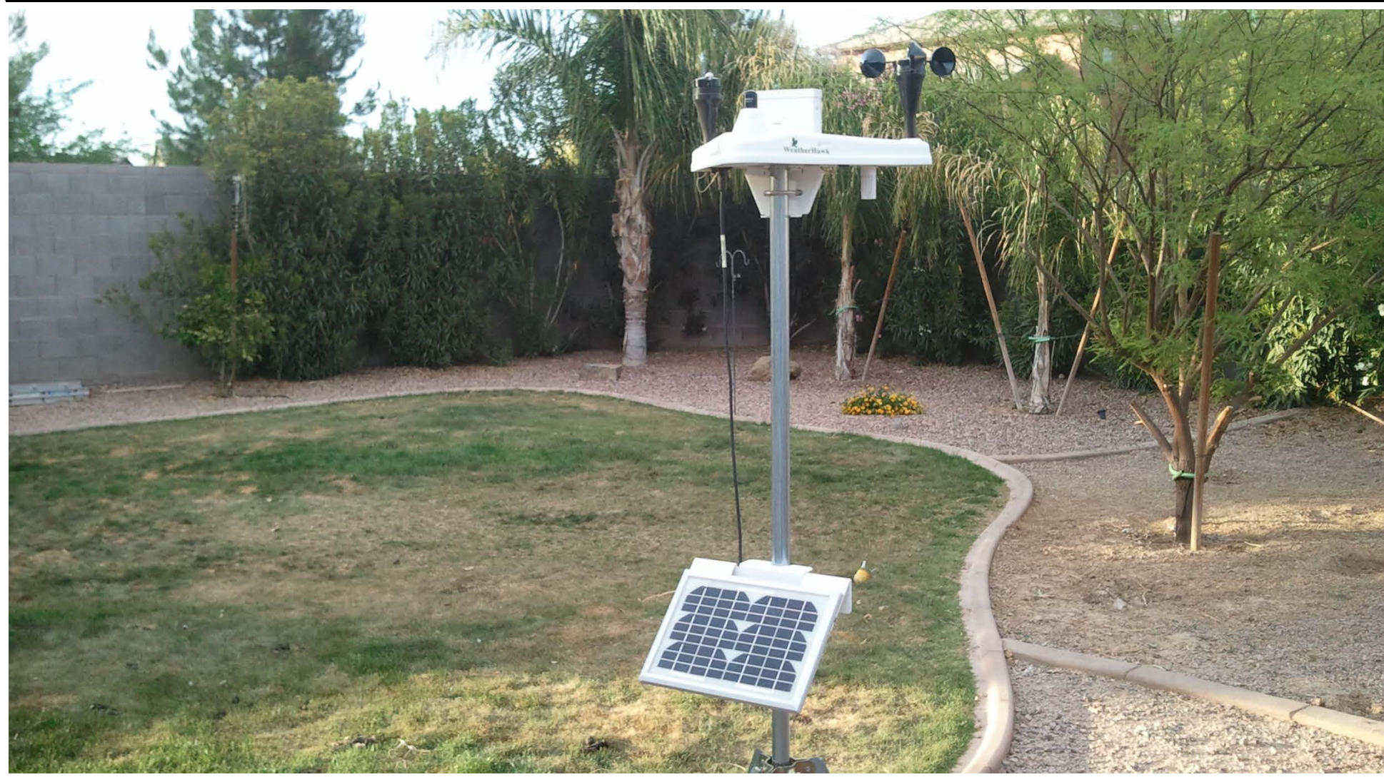
Fig. 2: WeatherHawk station sited at Station 4700. Each station measured hourly air temperatures, relative humidity, wind speed and direction, barometric pressure, and an evapotranspiration value derived from observed climate variables.
