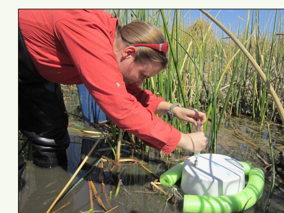
Fig. 5. Field placement of floating chambers on the shoreline (top), and gas sample collection (bottom).
