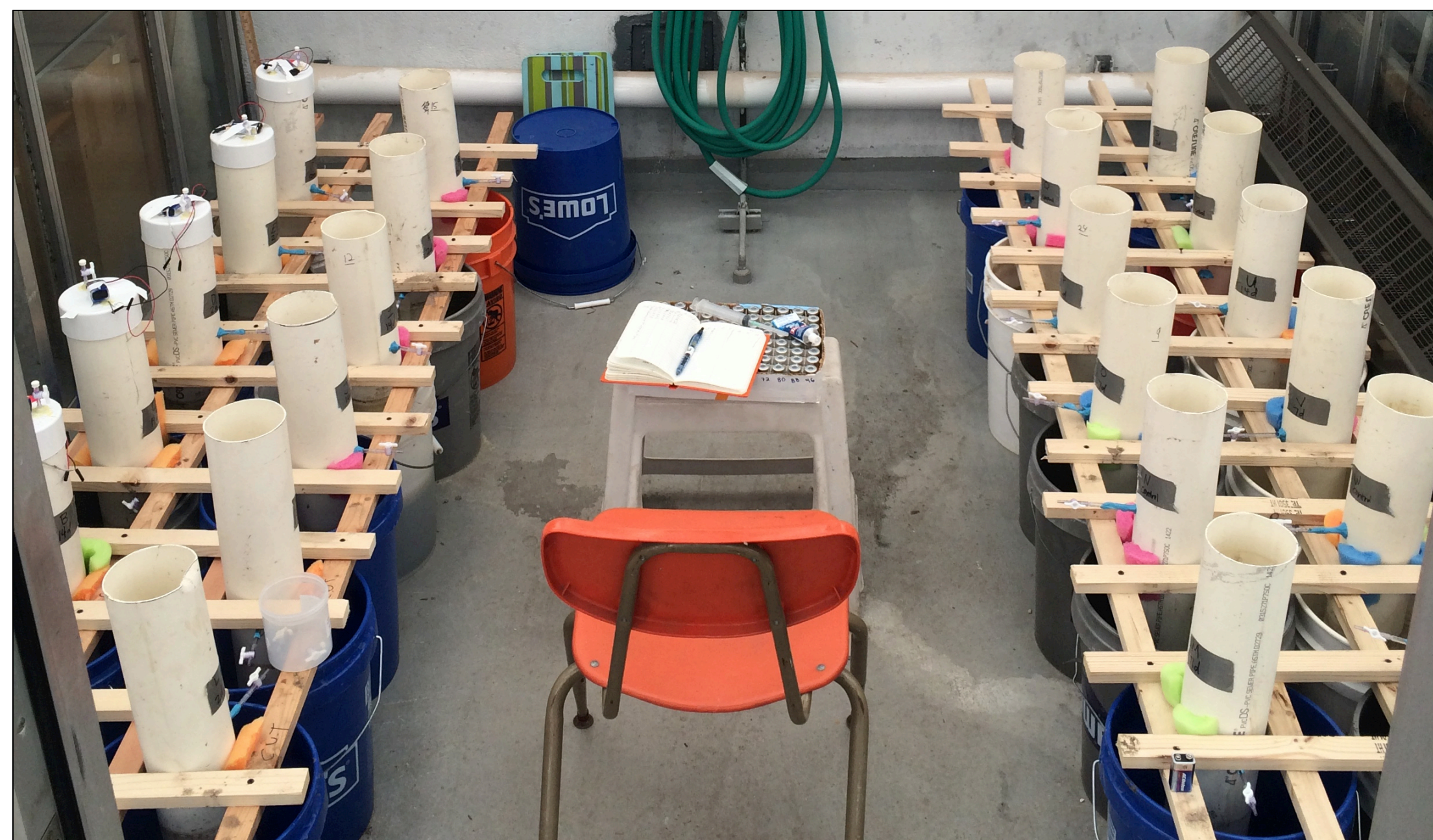
Figure 2. Experimental set up inside the greenhouse of the 24 wetland mesocosms.
