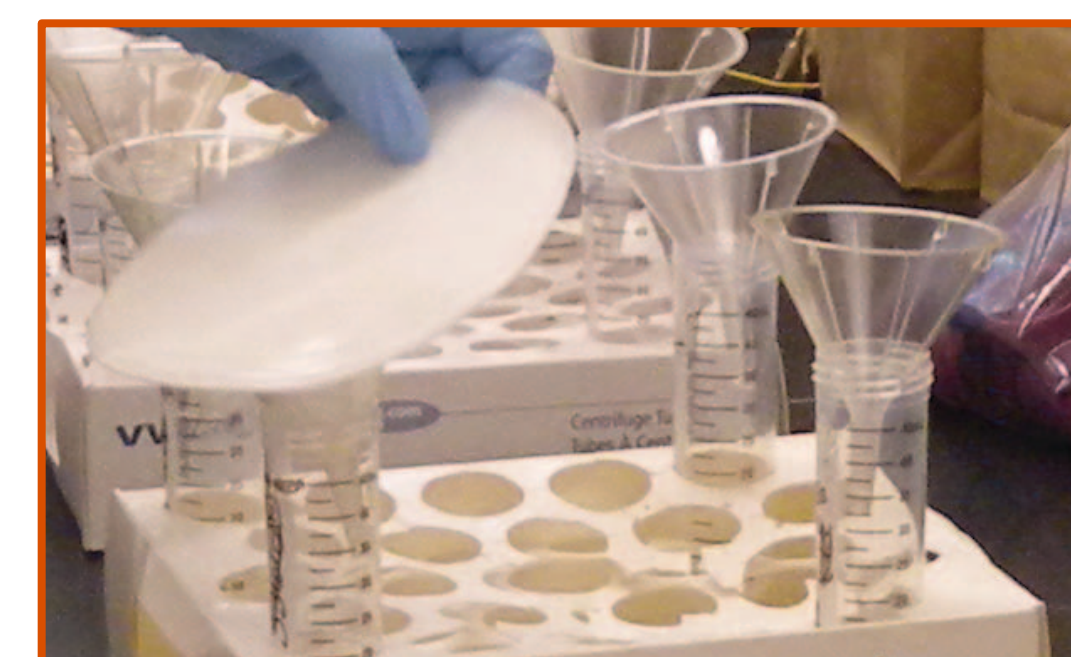
Nitrification potential extract filtration
