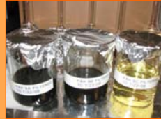
Fig. 2. Samples after ultrasonic solvent extraction.
