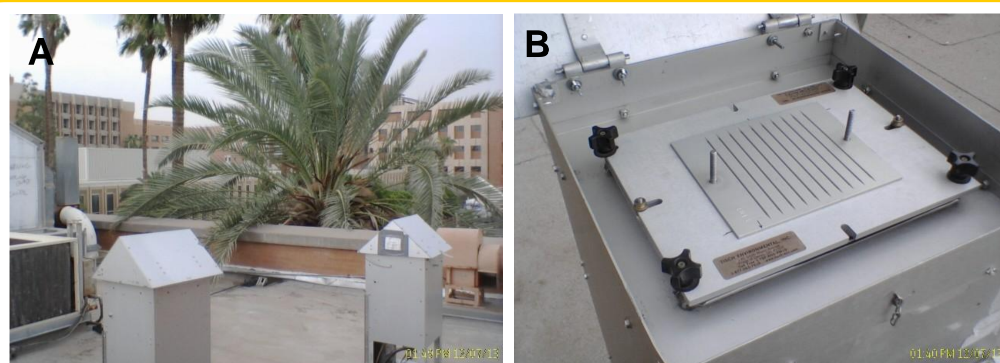
Figure 2 shows the Tisch high volume aerosol samplers (A) and the impactor plate (B) used in the collection of PM 2.5 and PM >2.5 aerosol samples collected at the ASU Tempe Campus on the roof of the Life Sciences A-Wing building.
