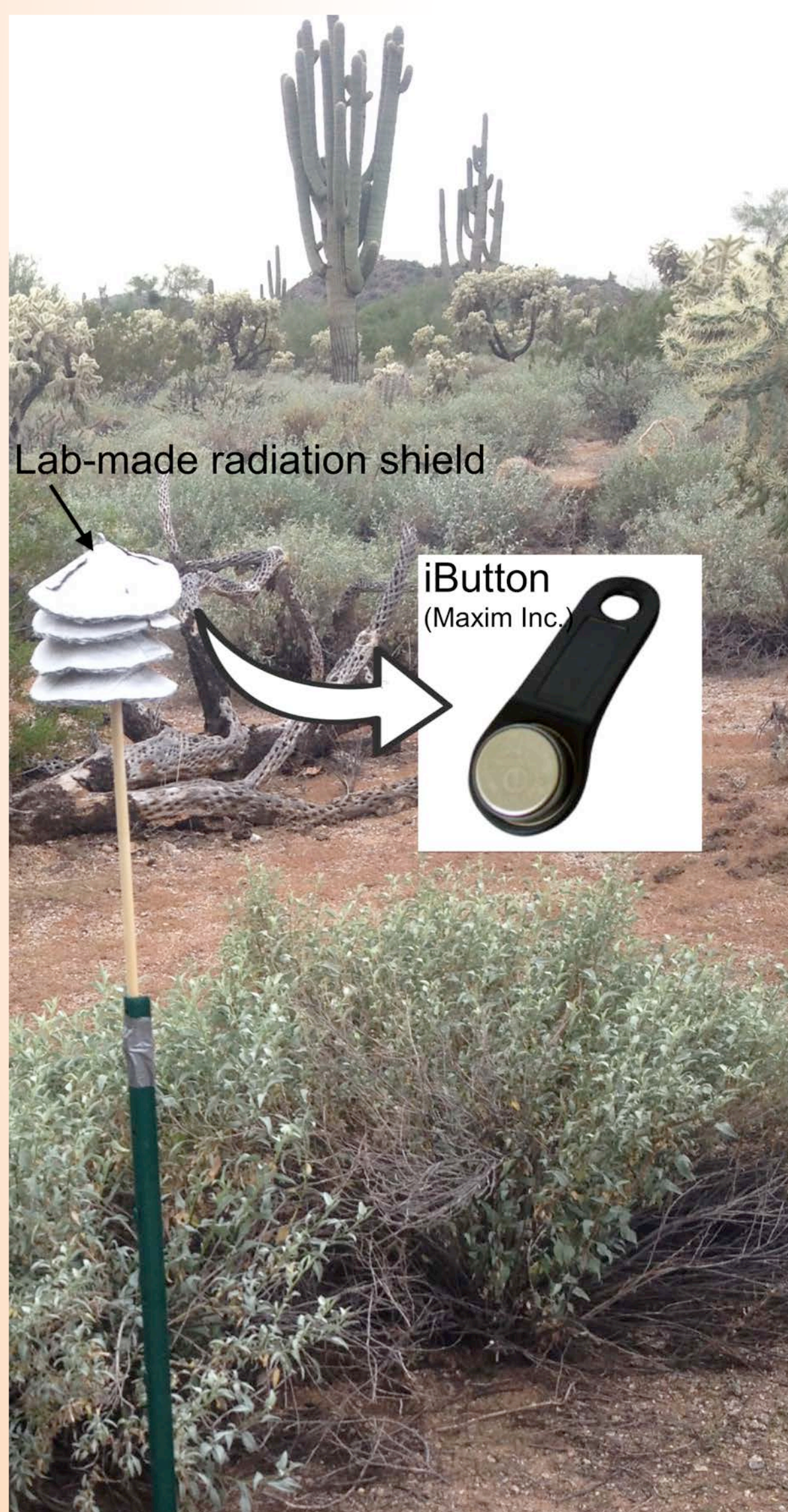
Figure 2. iButton deployed in a gill-style radiation shield at Utery Mountain park; a native habitat site (Sonoran Desert) in Phoenix, AZ.
