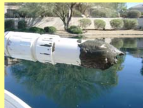
Figure 4: Lake coring device with protruding sediment
