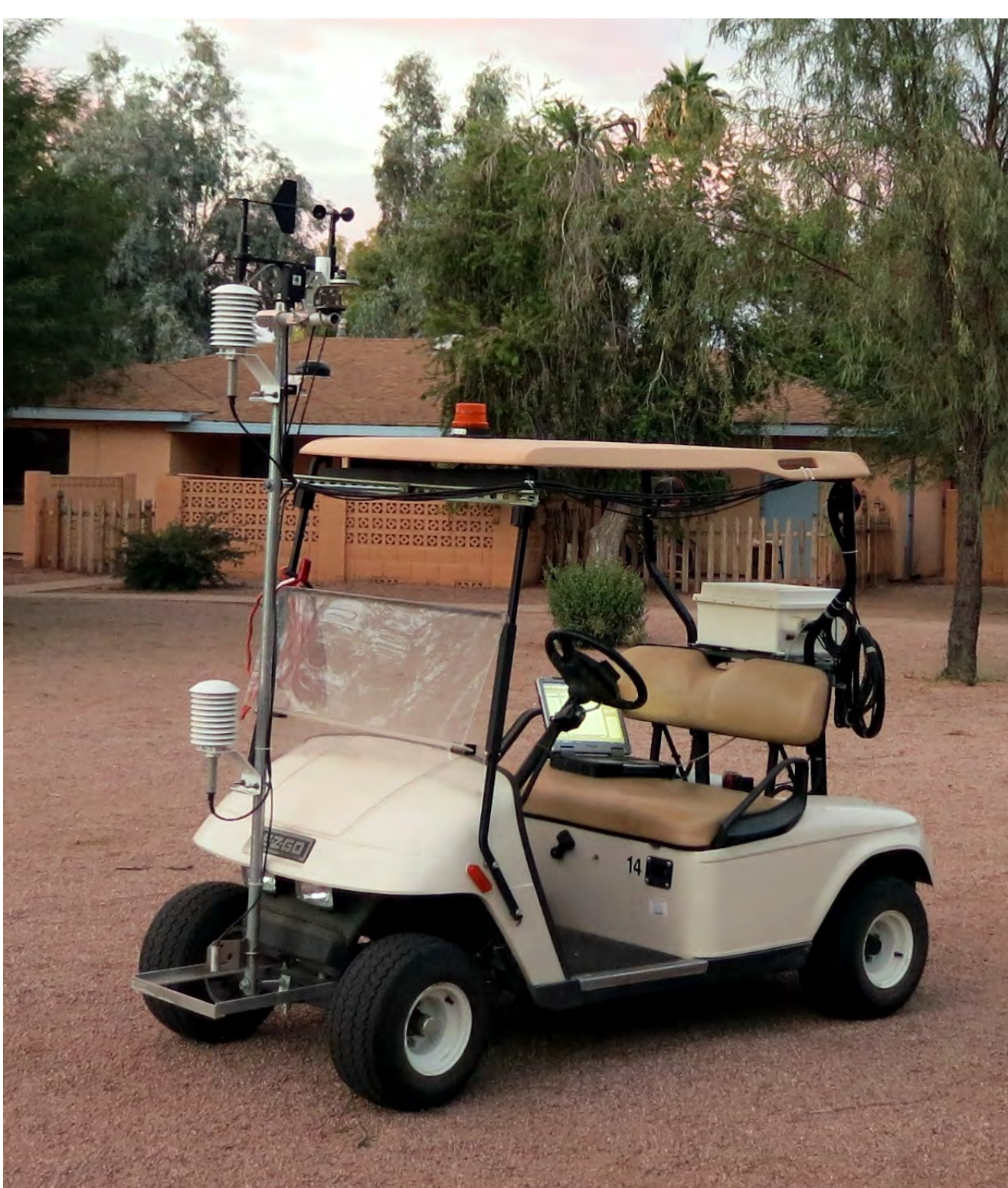
GOLF CART EQUIPPED WITH A GPS, SENSORS AND A DATA LOGGER
