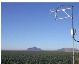
Sampling tower at the agricultural field site with a homogeneous fetch of 0.8 km. The tower height is 7 m and the mean crop height is 0.5 m. The mountain in the background is about 12 km to the west.
