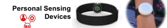
Heart rate monitors & UV dosimeters to assess the influence of microclimate conditions, design, & UV light on activity
