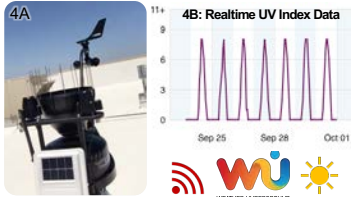
Fig 4: A) Davis roof weather station for local data & education, synced to Weather Underground; B) Realtime UV Index information.
