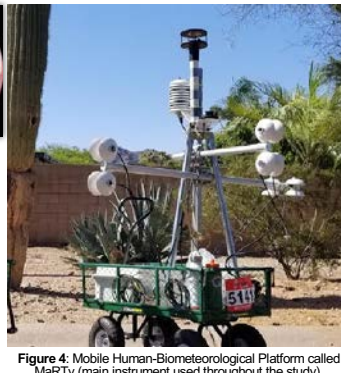
Figure 4: Mobile Human-Biometeorological Platform called MaRTy (main instrument used throughout the study).
