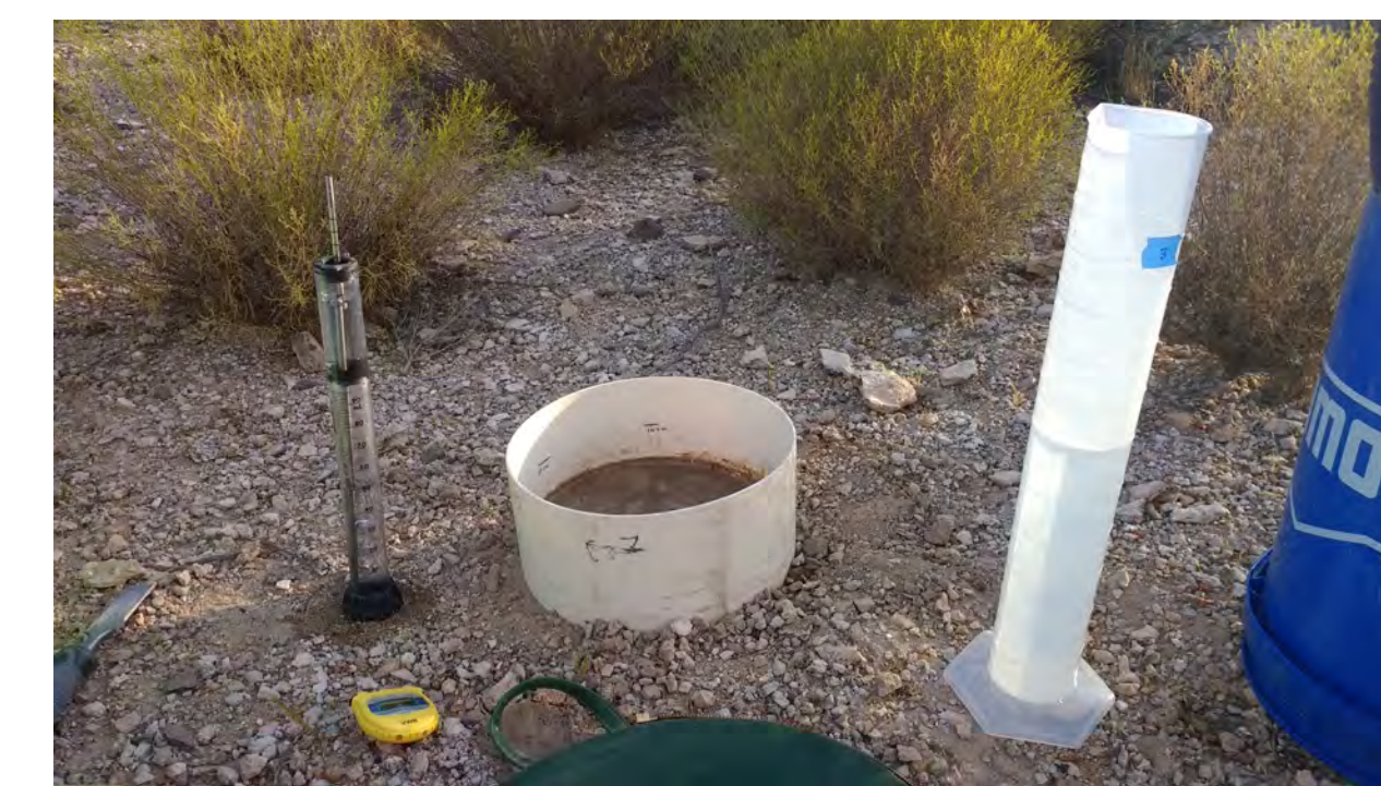
Tension infiltrometer for near-saturated infiltration rate
