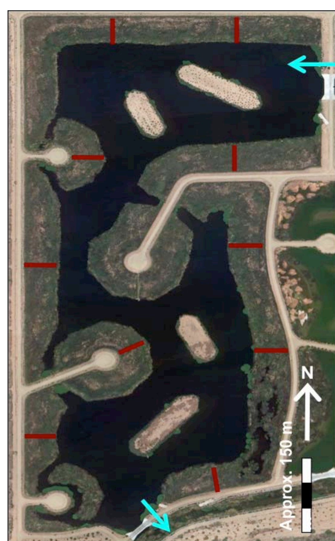
Figure 1. Constructed wetland study cell. Arrows indicate location and direction of inflow (top arrow) and outflow (bottom arrow) sites. Red lines indicate transect locations.
